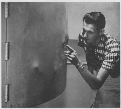
FLYING PIECES of a dummy component pounded these dents into the 1/4-inch steel protective plate surrounding the Livermore Laboratory centrifuge. Jack Workman (8121-1), centrifuge operator, examines the plate. The accident happened when the adhesive bond holding the component onto the centrifuge arm failed as the whirling arm reached a speed of 450 revolutions per minute.
